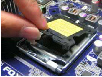
1. Remove protective socket cover.
