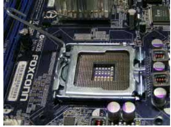
2. Release the CPU socket lever.
